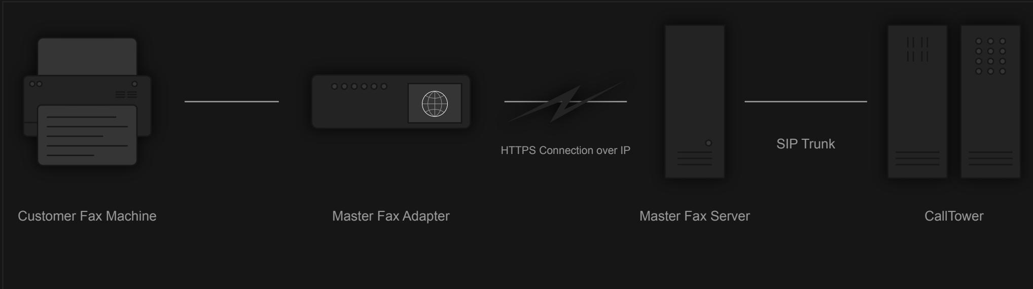
Rather than a traditional approach of requiring solid IP and a SIP connection all the way to the MasterFax Adapter, MasterFax replaces the link between the MasterFax Adapter and us with an HTTPS connection. This connection is not subject to the same concerns with jitter and latency as SIP, which provides reliable faxing over unreliable IP.
